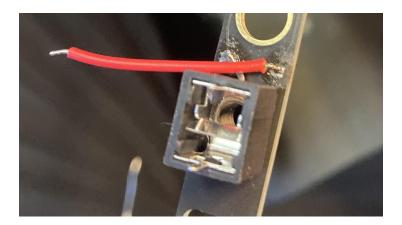
11. Use your soldering iron to heat the pad labeled "+" above your jack. Place the end of your wire on the pad so that it is soldered in place.
