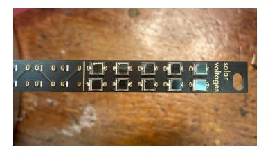
2. Stop after you have placed a few photodiodes and double check that they are all facing the right direction. We did 10 Photodiodes at once in this example, but 4-6 at a time is probably easiest.
