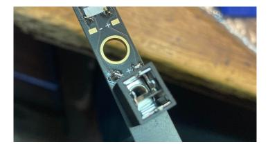
9. **Start with the Bottom jack**. Place the Thonkiconn in its hole so it sits in place and is relatively straight behind the PCB. Before you solder anything, use the knurled nut to secure the Thonkiconn jack to the PCB, ideally using a knurled nut driver tool. Solder the Ground pin directly to the pad labeled "-".
