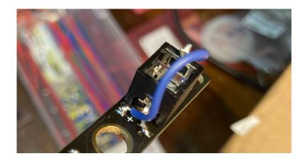
12. Solder the other end of your wire to the rear signal pin of your Thonkiconn jack, making sure the wire is well connected to both the pad and the jack. If you have a Multimeter, you can use it to test continuity between the two sides of each surface mount capacitor installed on the PCB.
