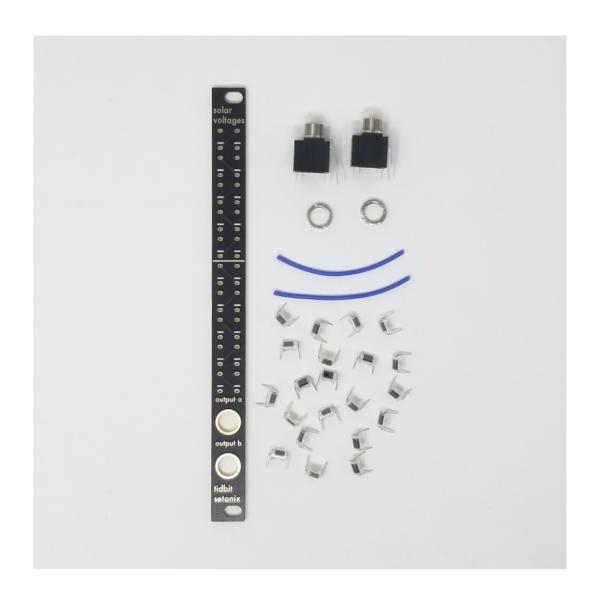
**Solar Voltages** Dual Light-Controlled Voltage Source - Eurorack Assembly Instructions - Eurorack (2hp)
