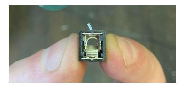
8. Prepare your first Thonkiconn jack. Bend the Ground pin towards the front of the jack and to the left as shown in the above picture. Clip it using your Edgecutters so it is about ¼" or 7mm long. It might also be a good idea to "tin" the Ground leg.
