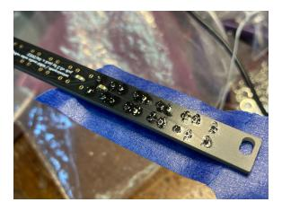
5. Solder the legs of every Photodiode. Make sure each pad has a good connection with enough solder, that you don't miss any, and that you don't mistakenly solder any pads that don't yet have Photodiodes placed!
