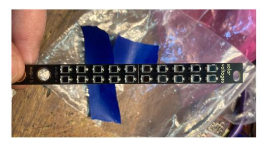
6. Repeat steps 2-5 until all the Photodiodes are soldered in place. When you're done, every Photodiode should be facing the same direction with the dot and line facing downwards.
