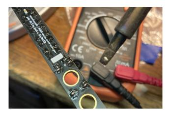
7. Use your soldering iron to "tin" the four pads near the bottom of the PCB labeled "+" and "-", coating them with solder.
