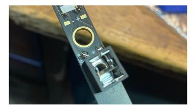
9. **Start with the Bottom jack**. Place the Thonkiconn in its hole so it sits in place and is relatively straight behind the PCB. Solder the Ground pin directly to the pad labeled "-".
