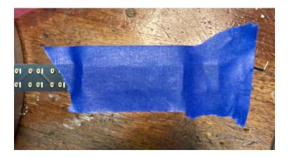
3. Place a strip of Painter's or Masking Tape over the photodiodes and stick the tape to the board on either side. This will hold the Photodiodes in place.
