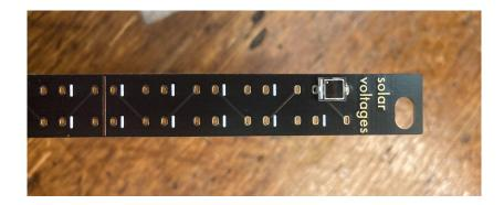
1. Place the PCB face up, holding it secure with a table vice or similar. Begin placing the Photodiodes in the appropriate footprints. Note that the Photodiodes are polarized! The side with the dot and line corresponds to the silkscreen line on each footprint. Each Photodiode must be installed facing the same direction, i.e. downwards if looking at the module head-on, in order for it to work.
