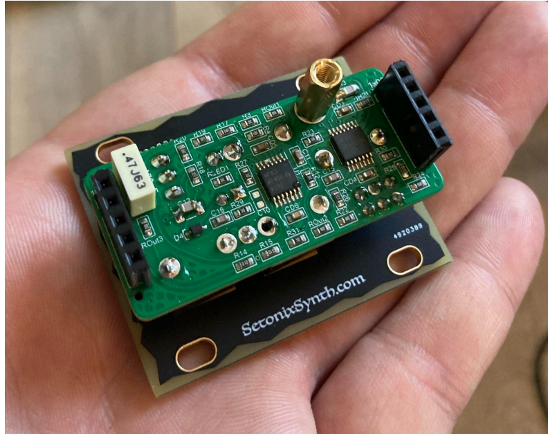
Rear of Panel PCB. Note the position of the 470nF cap and 11mm spacer.
